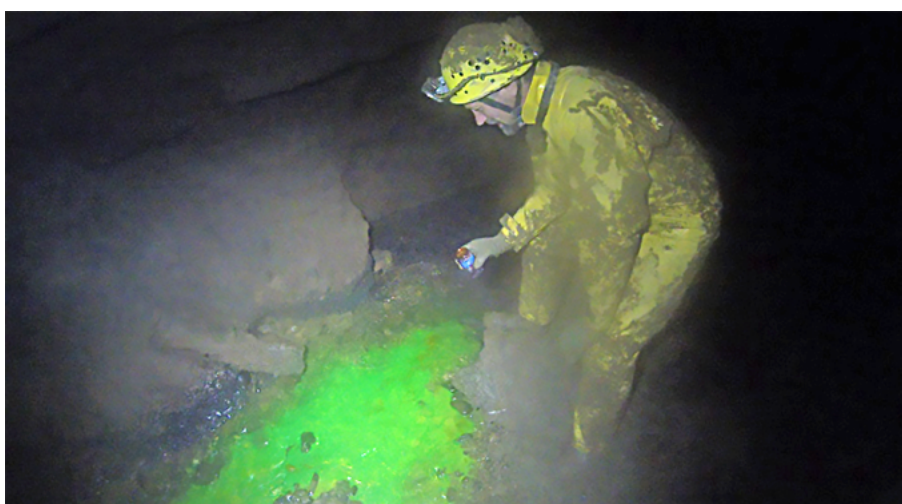
Pax releases a carefully calculated amount of fluorescein in Sesame
